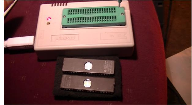
All you have to do is select the IC, load the ROM you dumped and press the "**Program**" button, which appears as
