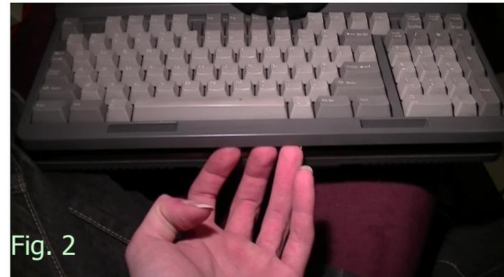
Place the keyboard carefully near the front of the machine, not so close that it kinks the ribbon but not so far that it stretches it.
